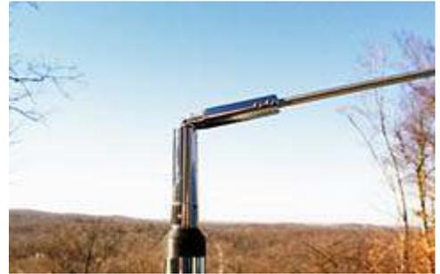
*Diamond NR22L antenna can be folded over by pulling up from the base.*
