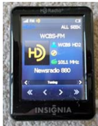
Insignia NS-HD02 portable radio tuned to WCBS-FM, 101.1 MHz. The HD2 subchannel carries WCBS-AM Newsradio 880.
