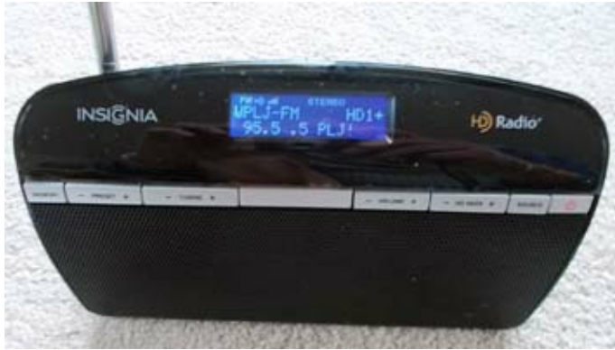
Insignia NS-HDRAD is a tabletop HD Radio with analog/digital reception on VHF – but no AM. [Pics by W2CH]
