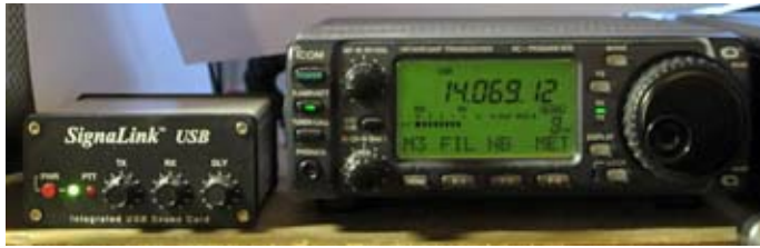
Signalink USB integrated USB Sound Card adapter (left) is connected to the Icom IC-706MkII transceiver for digital modes.
