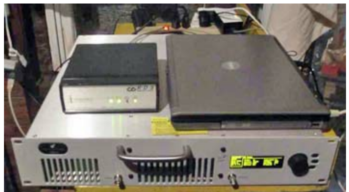
Current station equipment for WJZZ, 90.1 MHz FM. RDS encoder and Dell notebook computer are mounted on top of the Broadcast Warehouse TX600-V2 transmitter, which produces 175 watts RF output.
