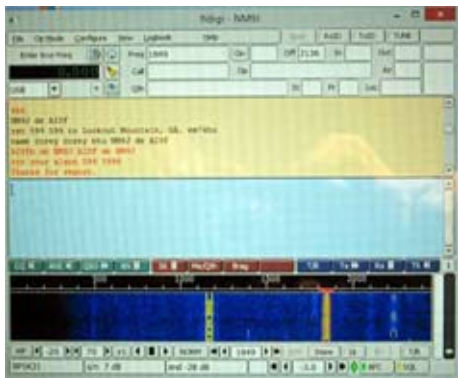
Fldigi software is shown, with several PSK31 signals visible on the waterfall display. Fldigi 3.21 is running on the Windows 8.1 desktop, on the HP X2 convertible notebook.
