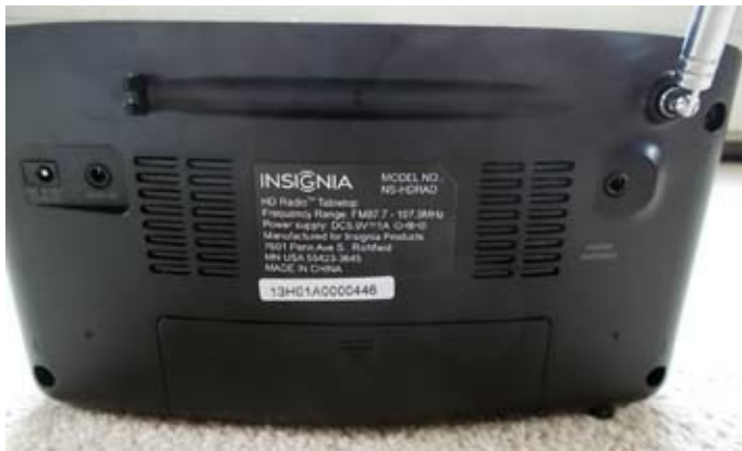
Rear of the tabletop radio. Connectors L-to-R are: external DC power, Aux-in and, on the right side, Pigtail antenna.
