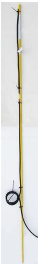
CFR dipole mounted on fiberglass driveway marker.
