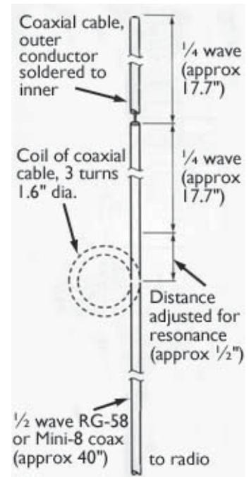
*Vertical CFR dipole antenna for the 2 meter band (146 MHz) as recently constructed.*
