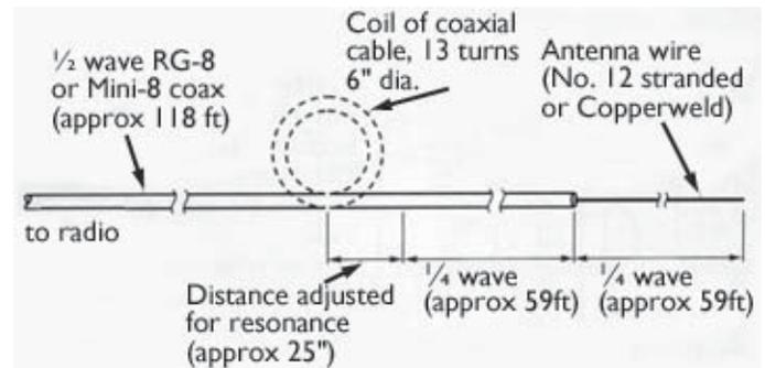
*RFD-1 horizontal dipole antenna for 80 meters (3.95 MHz) as described by W2OZH. Instead of a sleeve, there is a coil of coaxial cable, preventing current on the outer braid from traveling further down the coaxial cable.*
