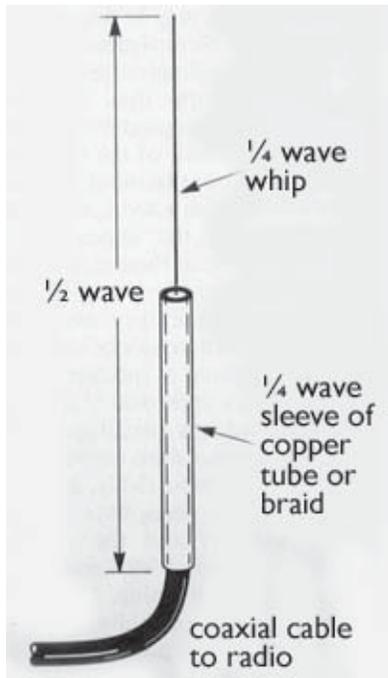
*Sleeve dipole consists of a half wave dipole whose lower element is a  $\frac{1}{4}\lambda$  metal sleeve surrounding the coaxial feeder cable.*
