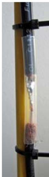
Detail of CFR dipole. Inner conductor of coax feeder is soldered to inner and outer conductors of top radiator.
