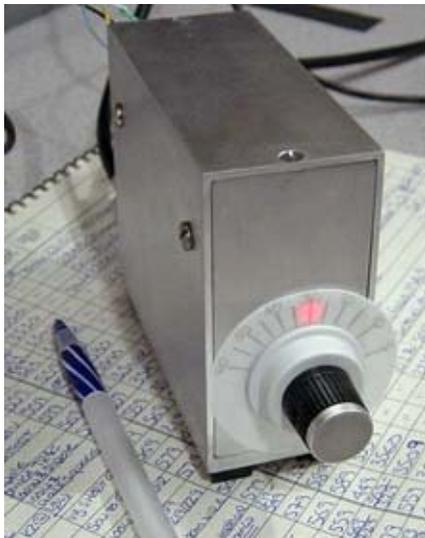
"Reggie" 1-transistor 80m transceiver.
