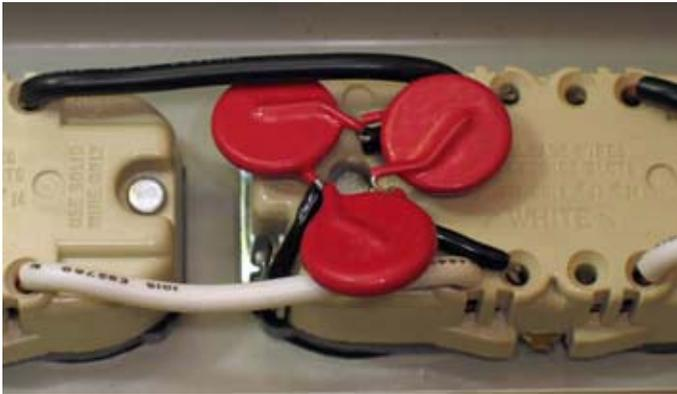
*This power strip contains three MOVs, or metal oxide varistors. The MOVs absorb electrical surges that exceed the normal 120 volts AC.*
