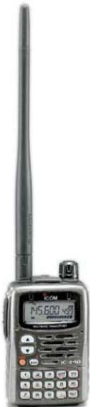
*Icom IC-E90 is one of the few modern transceivers that can be modified for 4 meter (70 MHz) operation.*
