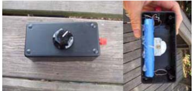
External ferrite loopstick antenna for use with Sony SRF-59 by Gil NN4CW.
