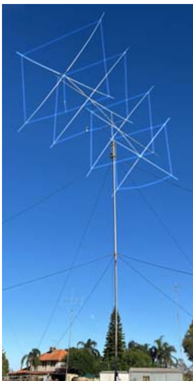
4-element cubical quad antenna built by Moz VK3CWB to a design by Jay NE2Q. Quad wires, boom and spreaders are emphasized for clarity. [VK3CWB pic.]
