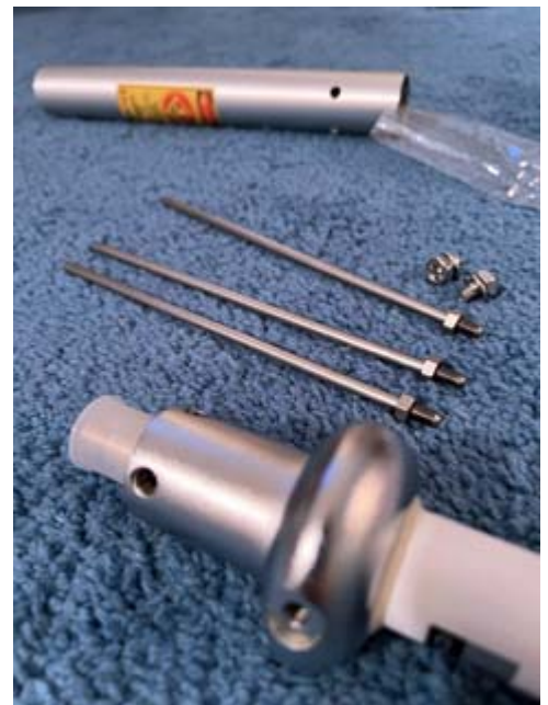
Base of Comet GP-3 antenna ready for the three short radials to be screwed in and tightened. [N2KZ pic.]
