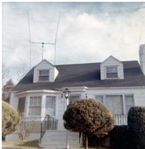
Jay NE2Q constructed this 20 meter cubical quad antenna at his father's summer home in Mohegan Lake. [NE2Q pic.]
