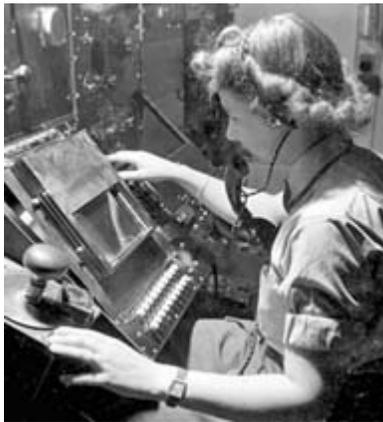
*WAAF radar operator plots aircraft on the CRT in a Chain Home Receiver Room. Her right hand has selected direction or height-finding and her left hand is ready to register the goniometer setting.*
