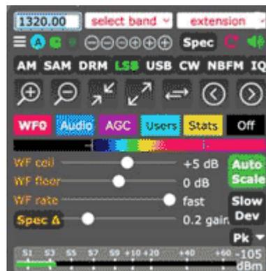
Kiwi SDR Control Panel set up to receive on 1320 kHz LSB. 'A' is the A/B VFO switch. Rotating red arrow is the clip 'record' button.
