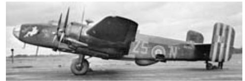
*Halifax bomber with H<sub>2</sub>S downward-looking radar mounted in the perspex cupola below Royal Air Force roundel.*
