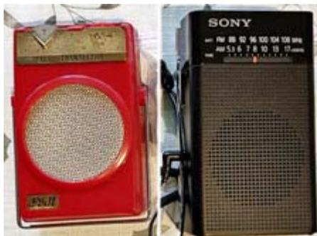
Radios old and new: two-transistor reflex left, Sony ICF-P26 right. [N2KZ pic.]
