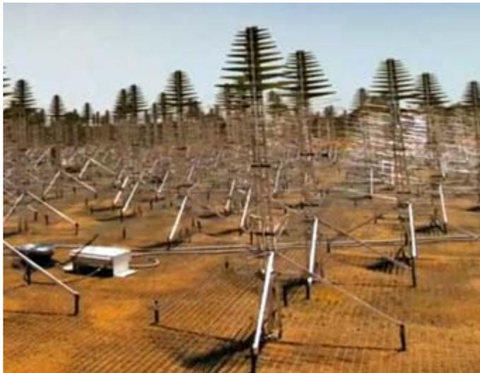
Crossed log-periodic Yagi antennas for 50-350 MHz beam upwarp from a ground plane in West Australia. [SKAO pic.]
