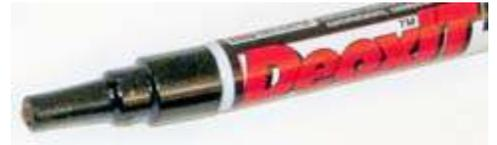
A well-used DeoxIT pen with a grimy, worn-down felt tip.
