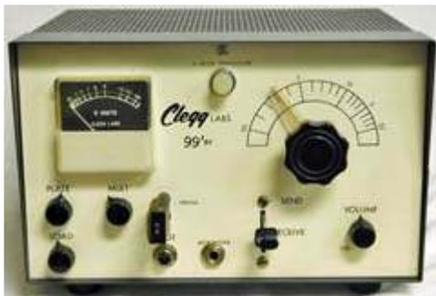
*Clegg Labs 99'er was an early 1960s AM transceiver for the 6 meter band.*
