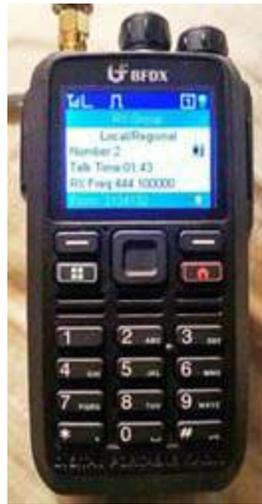
*Connect Systems' CS580 is an entry-level UHF DMR/FM HT suitable for amateur radio. This model is also available from KB Cubed in NJ.*
