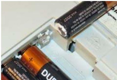
*Corroded battery contact as a result of electrolyte leaking from an AA-size cell.*
