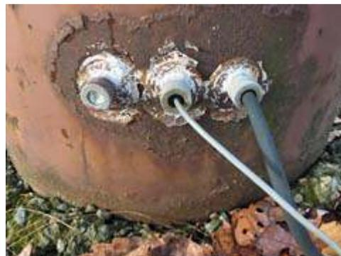
sitting above the batteries inside the oil drum. The now-empty third hole at the base of the drum was for feeding in the connection cable between the drum and the seismo-
