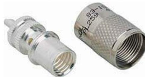
*Amphenol part number 83-1SP (PL-259) has a silver-plated brass body, nickel-plated brass coupling nut and a center contact pin made of silver-plated brass. The insulator is PTFE or LCP.*
