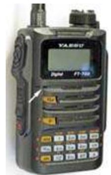
Yaesu FT-70D HT with microphone location arrowed.
