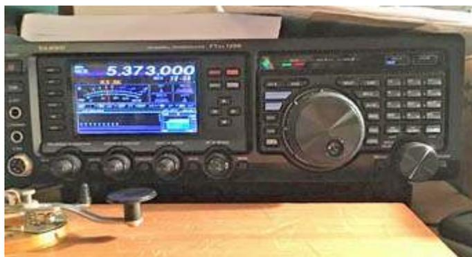
Yaesu FTDX1200 transceiver for 160 - 6 meters is capable of operating on 60 meters / 5.3 MHz. [N2KZ pics.]
