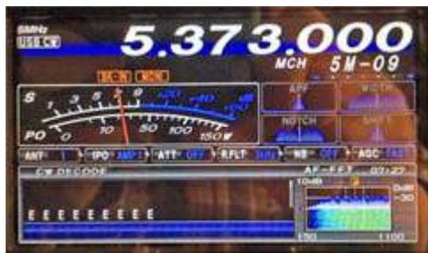
Close-up of FTDX1200 display, while in CW mode on memory channel 5M-09.
