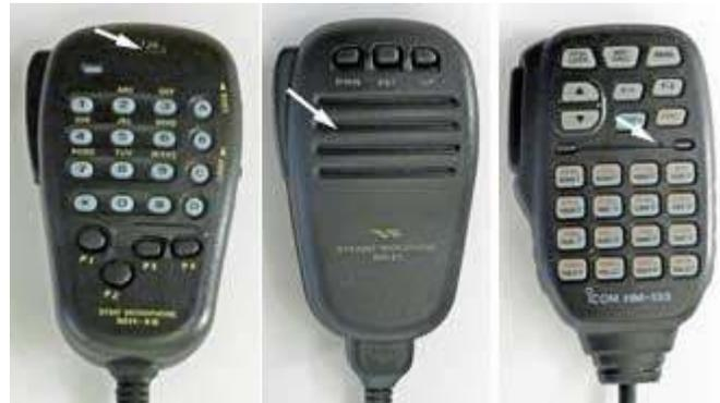
Three mobile microphones with location of the hole(s) for sound entry arrowed. L to R: Yaesu MH-48, Yaesu MH-31 (dynamic) and Icom HM-133.
