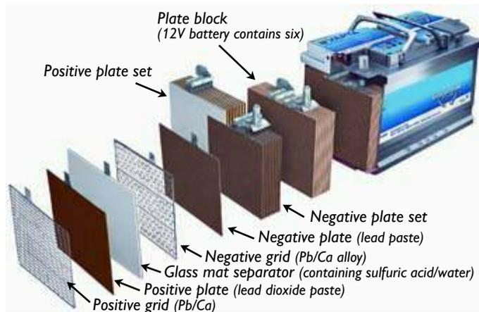
*Construction of an AGM (absorbent glass mat) sealed lead-acid battery [after SAE International].*
