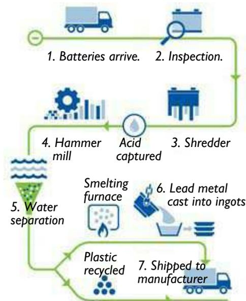
Lead-acid battery recycling process. [After DoeRun Company].
