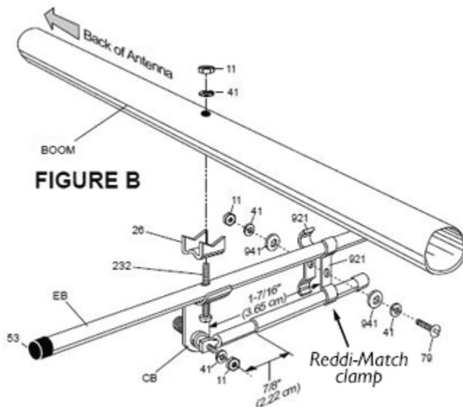
Picture from A449-6S Assembly Manual includes location of the "Reddi-Match" clamp (arrowed), shorting the adjustable gamma-match tube to the driven element.
