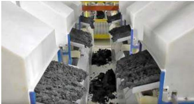
Six cells employing Aqua Metals' electrolytic process are shown recovering low-density lead from lead-acid batteries.
