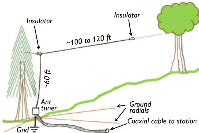
Sketch plan of an inverted-L antenna for 1.8 MHz. Overall wire length should be approximately 160 to 180 feet.
