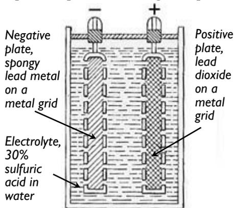
*Construction of one cell of a flooded lead-acid battery.*
