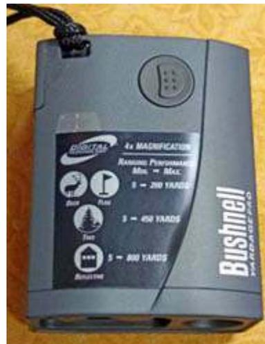
Bushnell Yardage Pro Sport Laser rangefinder has transmit and receive lenses plus monocular objective on front face. [KD2EVI pic.]
