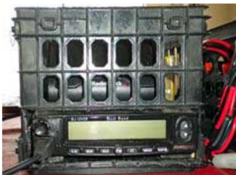
Plastic mini crate has hole cut for front panel of Lovji's Baojie BJ-UV55 dual band mobile transceiver. Loudspeaker is above.
