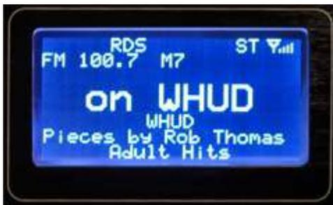
Typical display on HDT-20 LCD for an analog FM station with stereo and RDS.
