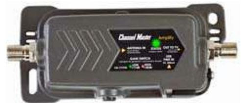
Channel Master 'Amplify'<sup>™</sup> adjustable-gain preamp covers 54 - 88 MHz and 125 - 700 MHz. Includes an FM trap for 88 - 108 MHz and a filter for LTE signals in the range 770 - 1000 MHz.
