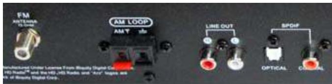
*Rear panel connections, L to R: F-type coaxial FM antenna socket, AM loop, RCA phonos for right and left analog Line Out, Optical SPDIF and coaxial SPDIF digital outputs.*
