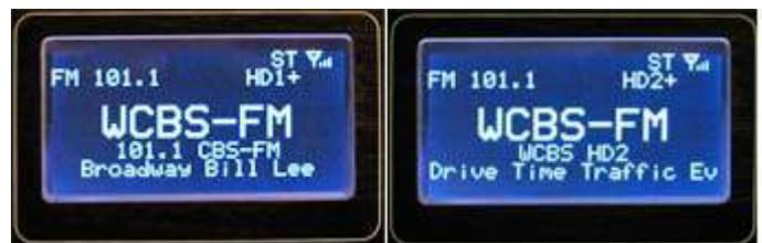
On the left, the steady ‘HD1+’ indicator shows that the first (HD1) multicast is being received, with additional multicasts available. On the right, ‘HD2+’ indicates that a second multicast has been tuned in — in this case WCBS-AM 880.
