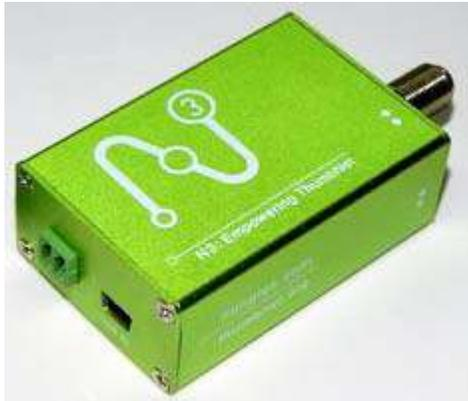
*ThumbNet N3 SDR is available in this custom aluminum case. External power and mini-B USB connectors visible at left.*
