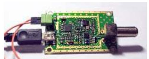
*ThumbNet N3 SDR receiver without RFI shield or custom aluminum case.*
