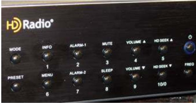
Front panel buttons on the HDT-20. In order to recall a stored memory channel you must first press “Preset”.
