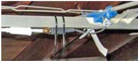
Secure the balun to the antenna boom with one or two cable ties.
