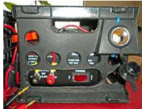
Second plastic mini crate contains Pyramid PS-8KX 12V DC power supply, with 12V DC accessory outlet attached.
