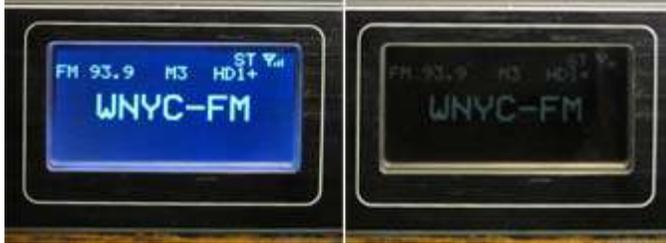
The backlight for the liquid crystal display (left) would switch itself off after a few seconds (right).
