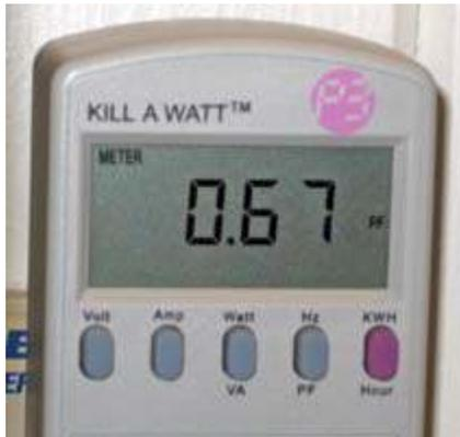
*Kill A Watt electrical consumption meter displays the power factor (PF) of a Philips 'Everyday' LED lamp.*
