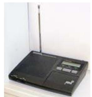
RadioShack SAME WeatheRadio suffered interference from nearby LED lamps.
