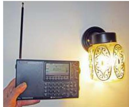
*Checking the RF interference from a Philips 'Everyday' LED lamp using a portable LW/MW/SW/FM radio.*
